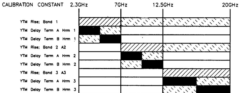
Figure 3-17a. Single-Band Delay and Risetime Compensation
