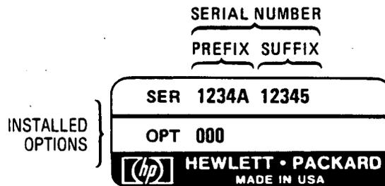
Figure i. Typical Serial Number Label
